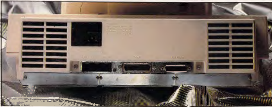
The I/O ports include three telephone sockets — two outputs and one input
